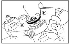
1. Spring preload adjusting bolt
